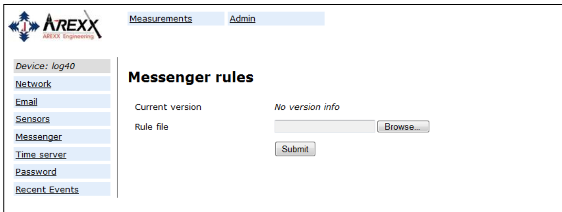
Figure 6: On this page of the BS1000 webserver you can upload the messenger rule file that defines the messenger rules to be applied on incoming measurements.
